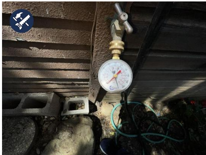
200 psi water pressure may burst the plumbing lines
